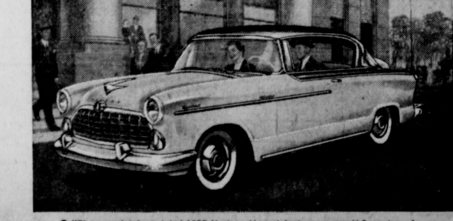
"The completely restyled 1955 Hudson Hornet features a new V-8 engine of advanced design, rated at 208 horsepower."
