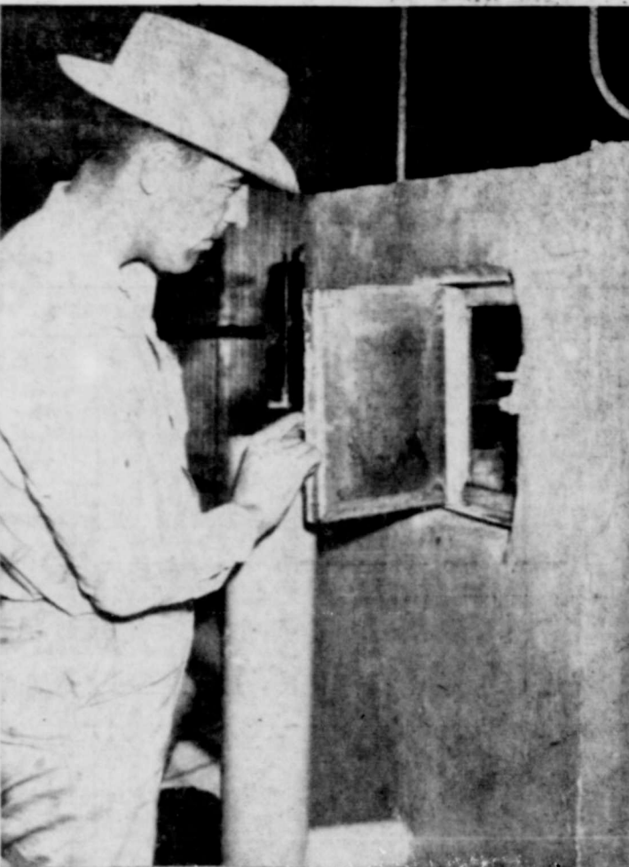
LUMBER YARD manager R. E. Williams is shown looking at heater of giant kiln at Valley Lumber Co. where lumber is dried completely in 72 hours. As much as 100,000 feet of lumber can be placed in kiln at one time. (Advocate Photo)
