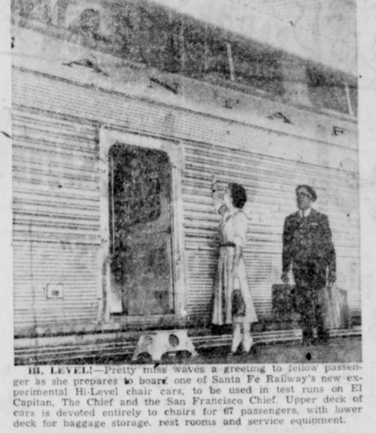
HI, LEVEL!—Pretty Miss waves a greeting to fellow passenger as she prepares to board one of Santa Fe Railway's new experimental Hi-Level chair cars, to be used in test runs on El Capitan, The Chief and the San Francisco Chief. Upper deck of cars is devoted entirely to chairs for 67 passengers, with lower deck for baggage storage, rest rooms and service equipment.
