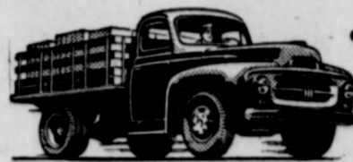
New Model R-130 Stake. Three light-duty stake models, 7 1/2 and 8 1/2-foot bodies. GVW ratings, 4,200 to 8,600 lbs. Famous Comfo-Vision cab.
