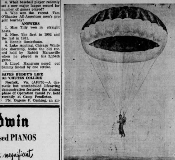
THE LATEST IN PARACHUTES is the Navy's new "extended skirt" type chute that will become standard equipment for pilots of jet and other highspeed planes in early 1950. The parachute, which has a 28-foot diameter, reduces the opening shock and gives a more stable descent to fliers who are forced to bail out of their fast-moving craft. (International)
