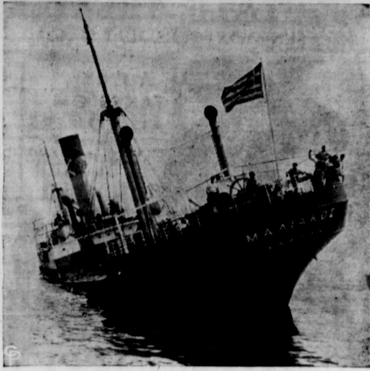
THE GREEK FREIGHTER Malakos lies with a dangerous list in Upper New York Bay after her cargo of coal shifted and almost caused her to capsize. A lighter and a tug later helped reload the cargo and the ship righted. The captain and the crew were taken off. (International)
