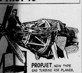
DOES DOUBLE JOB -18 THE PROPELLER AND ADDS POWER HROUGH A JET TO THE REAR. EXPERTS SAY ROPJET WILL POWER GIANT TRANSOCEANIC R LINERS OF TOMORROW. IT WAS DESIGNED SY GENERAL ELECTRIC ENGINEERS.
