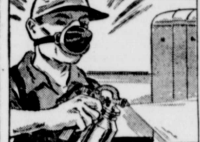
1. Not a gas mask, but a special nose mask to guard his breathing. It is worn by this spray painter at his job in one of the General Electric plants.
