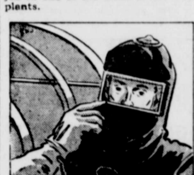
3. Frankenstein? No, just another G-E worker. His job is sandblasting big turbine castings for Uncle Sam's ships at one of the General Electric plants.
