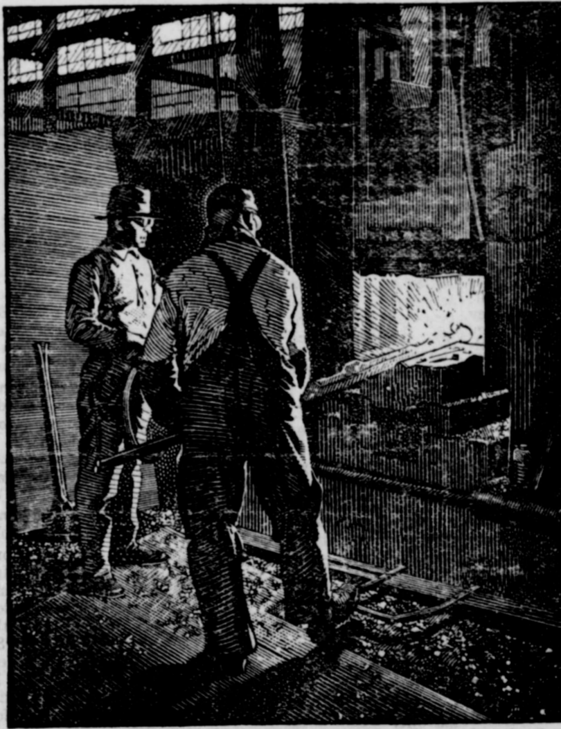
A scene in Chevrolet's great drop forge plant. A front axle is being forged from a bar of fine alloy steel.
