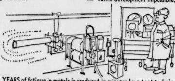
YEARS of fatigue in metals is produced in minutes by a test technique called "resonance bending" at Tube Turns, Louisville. Lengths of pipe are set to vibrating several thousand times a minute, simulating stresses normally occurring only after years of service. The pipe shakes itself until it cracks from fatigue. The method makes it possible for engineers to determine the probable lifetime of pipelines.
