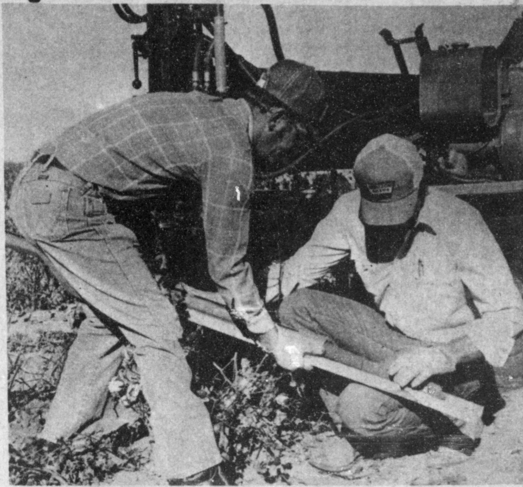
PULLING CORE SAMPLES --Dan Seale and "Shorty" Lancaster pull a soil core sample at a Bailey County moisture survey site. The samples are then measured to determine available soil moisture and amount needed to bring it up to planting standards.
