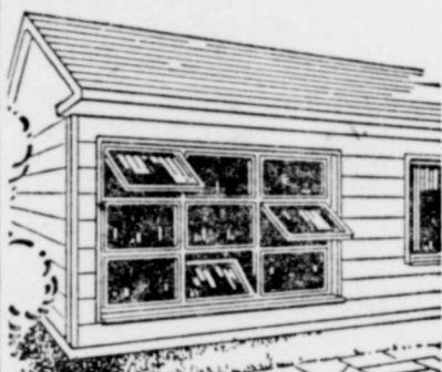
Attached garage, top, can become new living space for a growing family with a minimum of remodeling, bottom. Here the garage door was replaced by a wall of awning and hopper windows of ponderosa pine.
