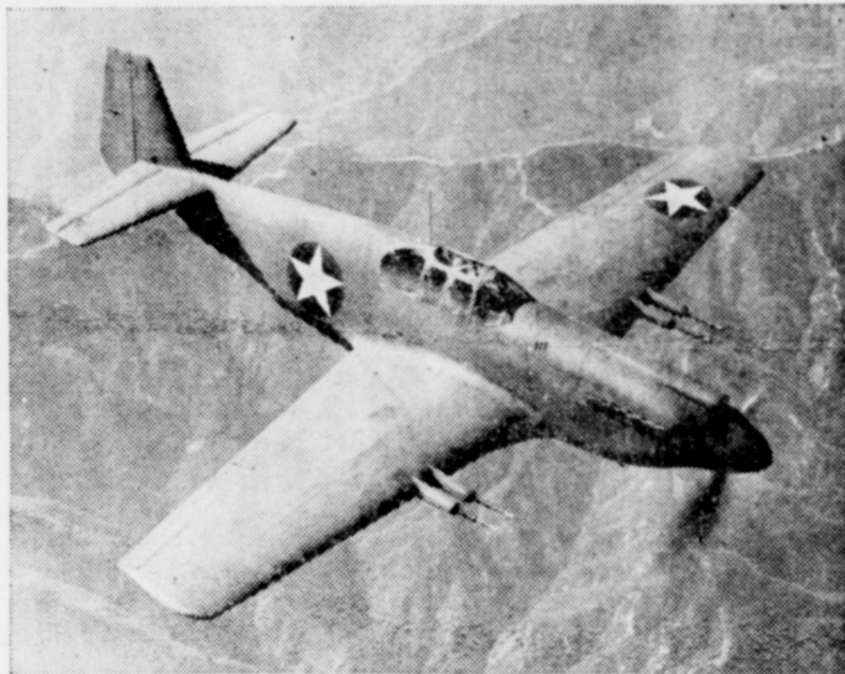
Four 20-millimeter cannon have made the North American P-51 Mustang fighters, similar to the one shown above, the scourge of Axis transportation. On land and sea, Mustangs have won the nickname of "train busters" for their record in destroying scores of enemy locomotives in occupied Europe.
