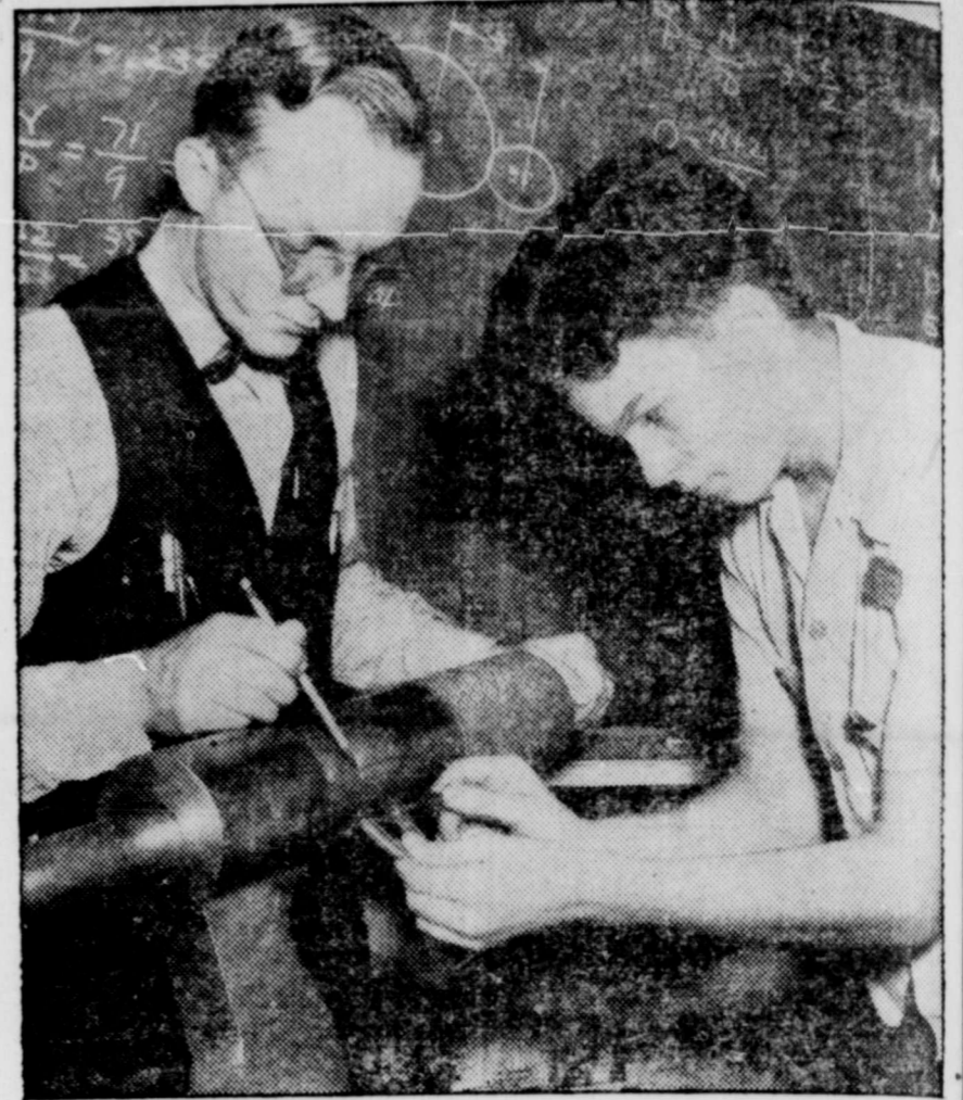
Many unique methods of instruction are used at the Henry Ford Trade School in Dearborn, Mich. For example, this photo shows an instructor in shop theory explaining the operation of a micrometer by utilizing a giant model built specially by Trade School students as a practical classroom aid. In his hand the young student holds a small micrometer he uses in the Trade School shop. This school, now supplying hundreds of graduates to important jobs in defense industries, has just celebrated its 25th birthday. It was founded in 1916 by Henry Ford to teach trades to boys. The school is located in the heart of the vast Ford Rouge plant.
