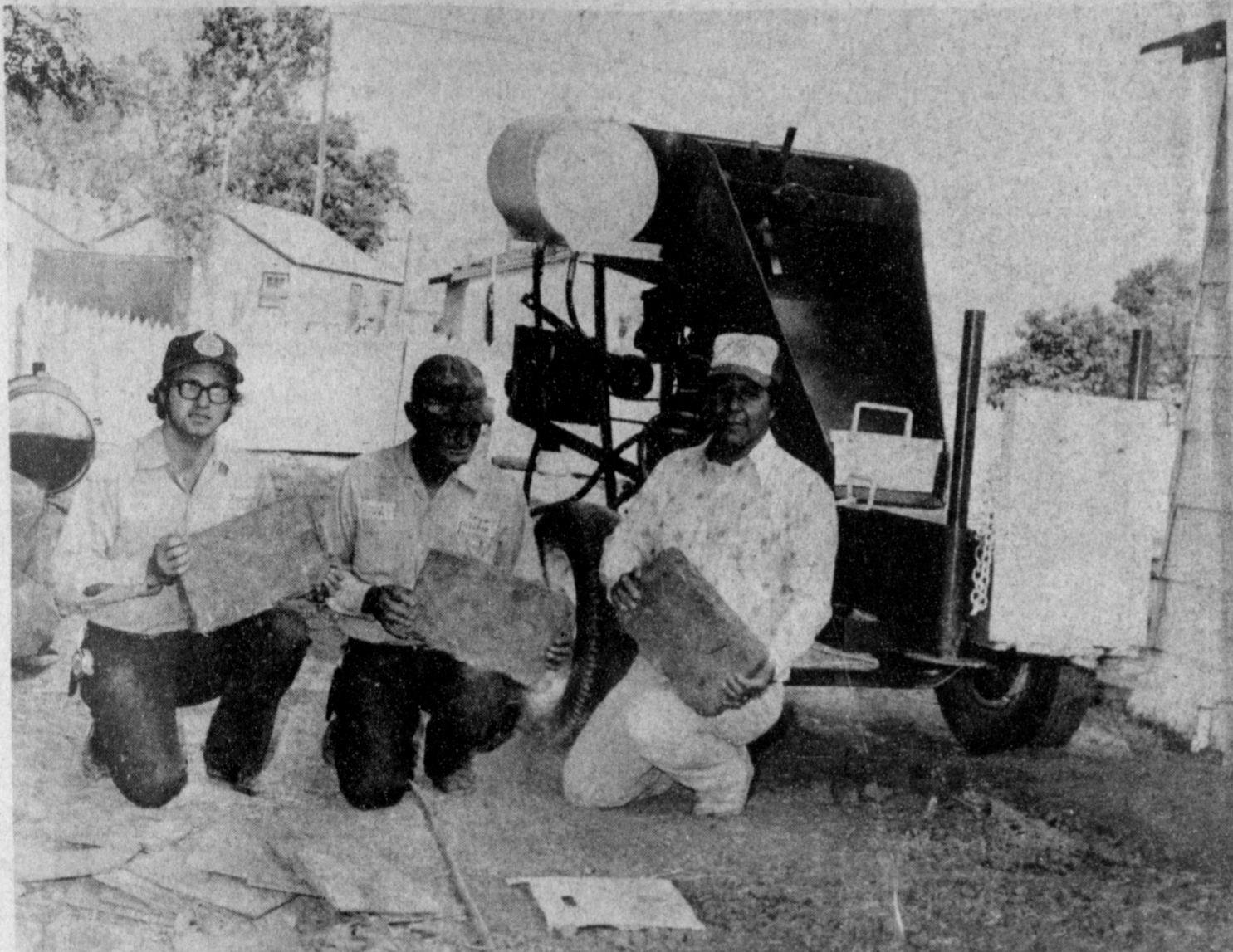
ADOBE BRICK MACHINE INVENTORS... In the background is a new machine which inventor Nick Manzanares expects to help reduce some of the soaring costs of heating and cooling homes and businesses. The machine produces adobe bricks, which formerly were made by hand. Holding some of the 4x10x14 bricks produced by the machine are from left, Keith Harp, Edd Harp and Manzanares. The portable machine will make 2-4 bricks per minute, and will be available for the construction of new facilities. Manzanares said the inside temperature in an adobe building is 18-20 degrees cooler, without air conditioning, than the outside temperatures.
