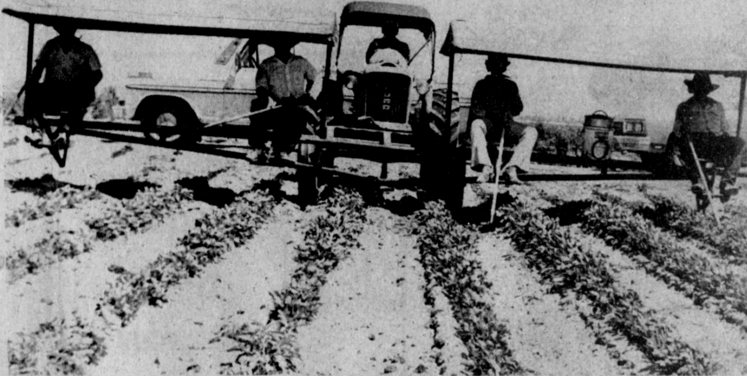
INVENTION HELPS IN HOT WEATHER... Lewis Scoggin has invented a new machine which not only cuts down on fatigue from the extreme heat, but cuts time from approximately four days to one day to clear weeds from his fields. Here, he and his chopping crew are shown as they get ready to go down a few more rows in the peanut field in the West Camp Community. His base is a spray rig, with swivel seats, canopies and foot braces.
