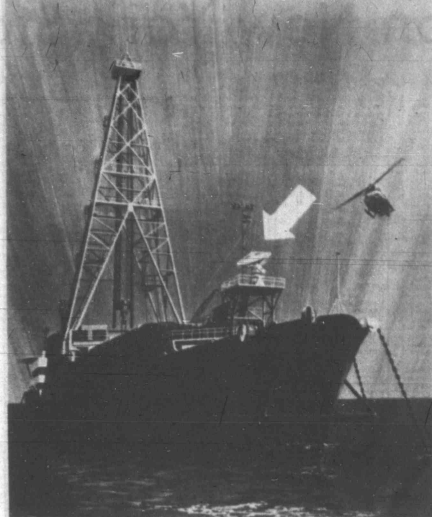
A communications system which makes use of an outer space satellite will be installed on vessels which conduct offshore exploratory drilling for Exxon Co., U.S.A., as shown in this artist's drawing, providing instant rig-to-shore contact.
