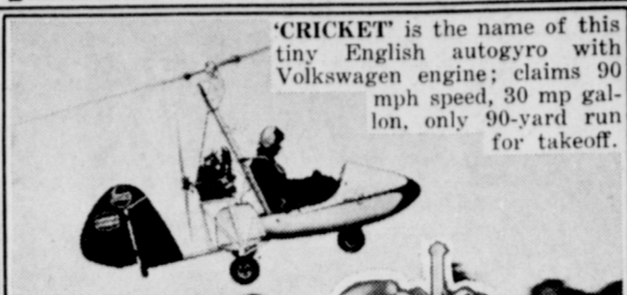
'CRICKET' is the name of this tiny English autogyro with Volkswagen engine; claims 90 mph speed, 30 mp gallon, only 90-yard run for takeoff.
