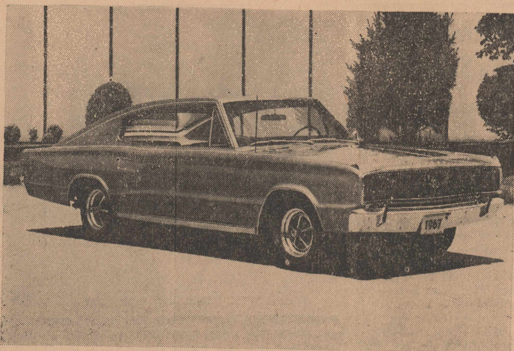
THE 1967 DODGE CHARGER features new fender-mounted turn signal indicators as an exterior change, and has an improved, console-free rear seating area, along with an optional front seat fixed center cushion and fold-down arm rest to make room for a third passenger in the front.
