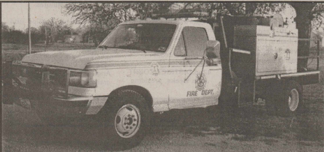
COTTONWOOD'S NEW FIRE TRUCK—A 1988 Ford F350 with a 400 gallon water tank, hose reel and firefighting equipment.
