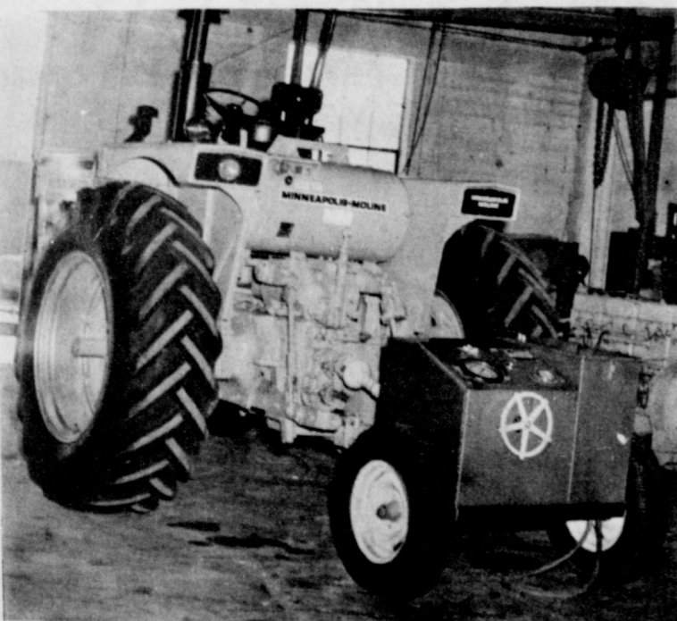
Above and below: Dynamometer for checking performance and H. P. on all types of farm tractor and power units up to 250 H. P.
