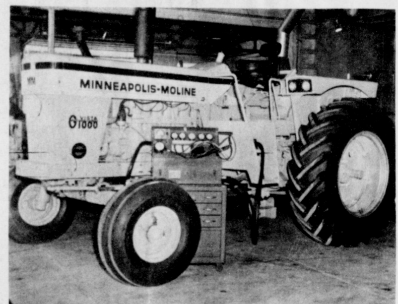
Hydro analyzer and testing equipment to check our hydraulic pumps-flow and volume and all types of hydraulic lifts.
