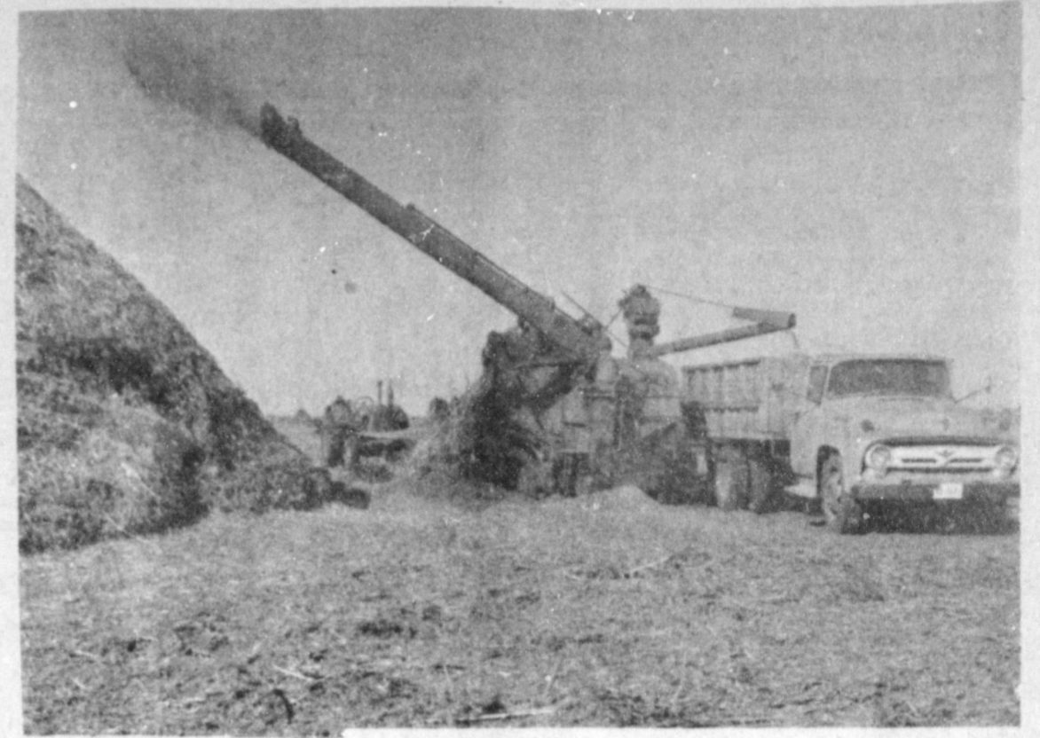
SEPARATOR---This case separator is one of the last of its kind used in the Muleshoe area. The Brown brothers, Dee and Jackie, farm 10 miles north of Muleshoe and this operation on their farm is the threshing of cat tail millet. Carried on a conveyor belt, the bundles travel to the machine, the grain pours into the truck and the blower spouts straw into a stack beside it. They harvested 600 acres.
