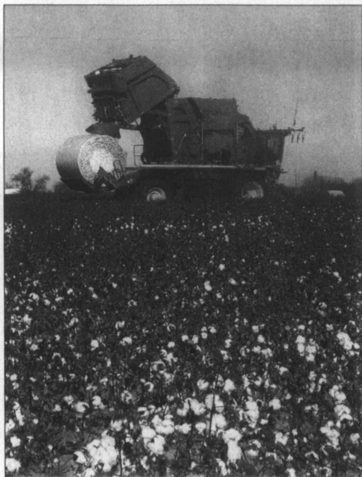
Round bale cotton ... In this field just north of N. 8th Street in Tahoka, the cotton is stripped and wound into round bales, instead of the usual cotton modules, ready to take to the gin. (LCN PHOTO by Gary Jones)
