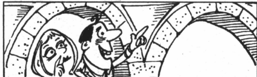
The triangular area between the sides of two adjacent arches is called a spandrel.
