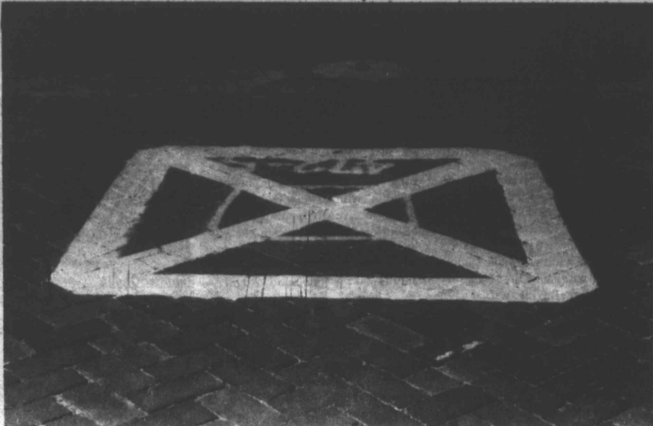
"X" MARKS THE SPOT - No, there's no buried treasure underneath city streets in Tahoka, but someone has painted numerous X's on the streets here. According to a spokesperson for The Texas Department of Transportation, the X's are reference points for an aerial survey to be conducted in the future. News personnel tried standing on them and saying "Beam me up, Scotty!" but, after nothing happened, hastened back to the News Office to work on this week's issue.
