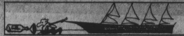
A ship model in a bottle is first constructed outside the bottle. The builder then folds the masts down, slides the ship down the bottle's neck and pulls up the masts with a thread.
