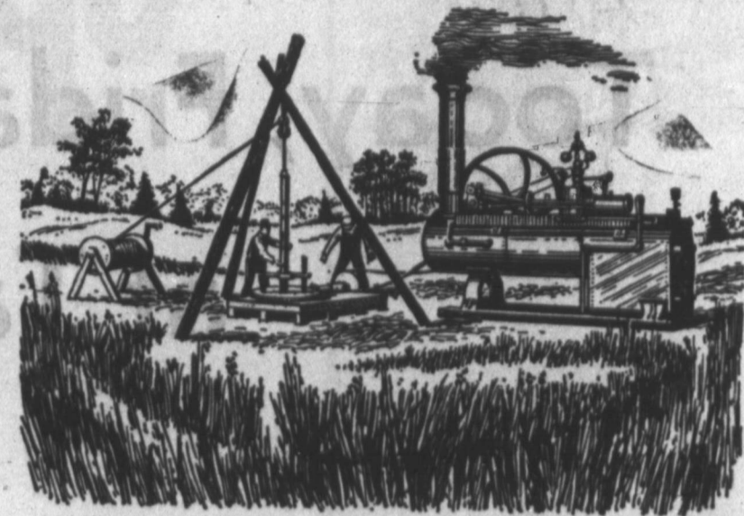
EARLY RIG —Based on historians' reports, this is an artist's interpretation of the type of steam-powered device that Tol Barret used to drill the first Texas oil well in 1866. It reportedly employed the principle of today's rotary rig which bores a hole in the earth. In contrast, the cable tool, commonly used in many early wells, drilled a hole with the up-and-down motion of a bit suspended on a cable or rope.
