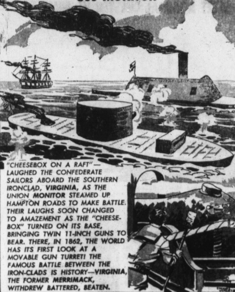
"CHEESEBOX ON A RAFT" — LAUGHED THE CONFEDERATE SAILORS ABOARD THE SOUTHERN IRONCLAD, VIRGINIA, AS THE UNION MONITOR STEAMED UP HAMPTON ROADS TO MAKE BATTLE. THEIR LAUGHS SOON CHANGED TO AMAZEMENT AS THE "CHEESEBOX" TURNED ON ITS BASE, BRINGING TWIN 11-INCH GUNS TO BEAR. THERE, IN 1862, THE WORLD HAS ITS FIRST LOOK AT A MOVABLE GUN TURRET IN THE FAMOUS BATTLE BETWEEN THE IRON-CLADS IS HISTORY—VIRGINIA, THE FORMER MERRIMACK, WITHDREW BATTERED, BEATEN.
