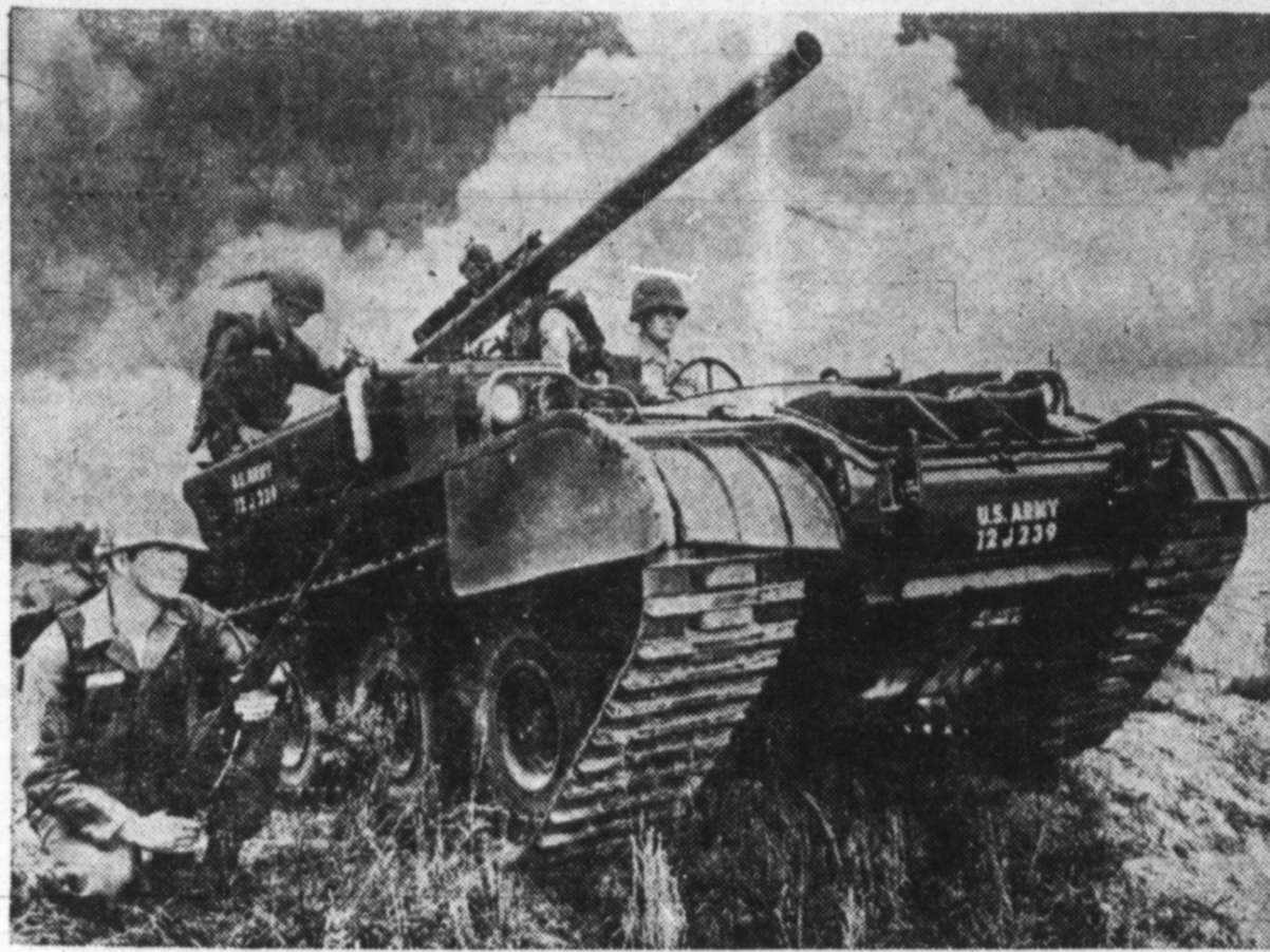
VERSATILE WEAPONS PLATFORM—This multi-purpose tracked Army vehicle mounting a 106mm recoilless rifle was originally designed to carry—and does—a 90mm anti-tank gun. Dubbed "Scorpion," it just as easily carries a 4.2-inch mortar or four machine guns.
