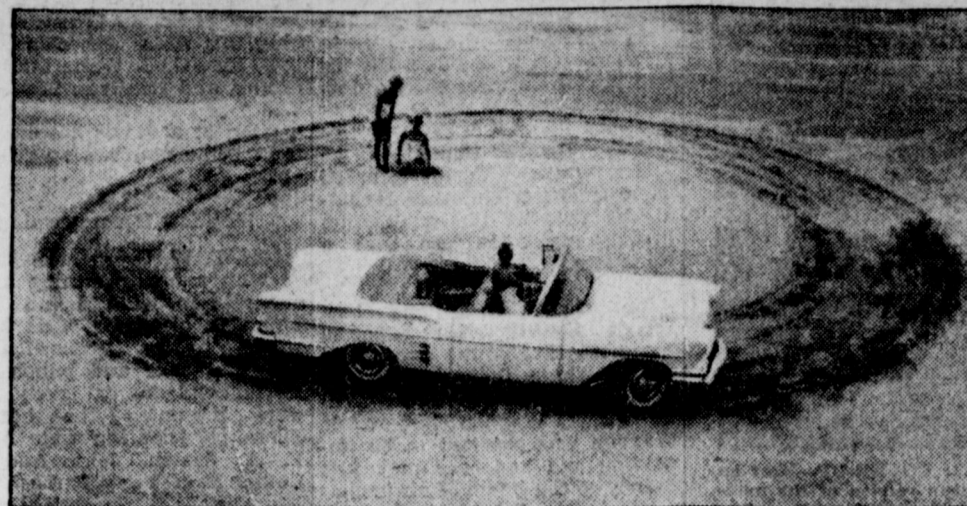
Around and around she goes and where she goes proves to be a perfect circle in the sand. Continued refinement of Chevrolet steering permits tight turns in an area 2 1/4 feet less in diameter than previous models, despite a two-and-one-half-inch increase in the car's 1958 wheelbase.
