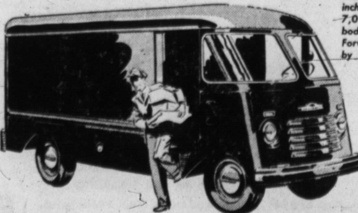
LIGHT-DUTY DE LUXE PANEL* Model 3105—116-inch wheelbase, Maximum G.V.W. 4,600 lb. Also available in Medium-Duty model 3805—137-inch wheelbase, Maximum G.V.W. 6,700 lb.
