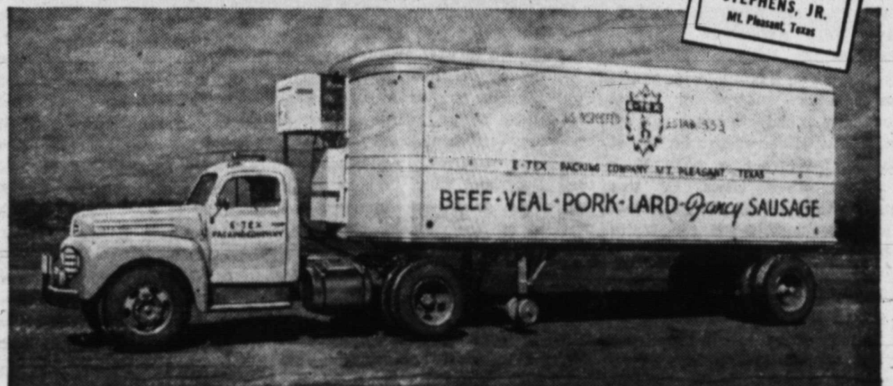
Ford 145-horsepower Model F-7 BIG JOB shows Gross Combination Weight rating of 35,000 lbs. as a tractor; Gross Vehicle Weight rating of 19,000 lbs.
