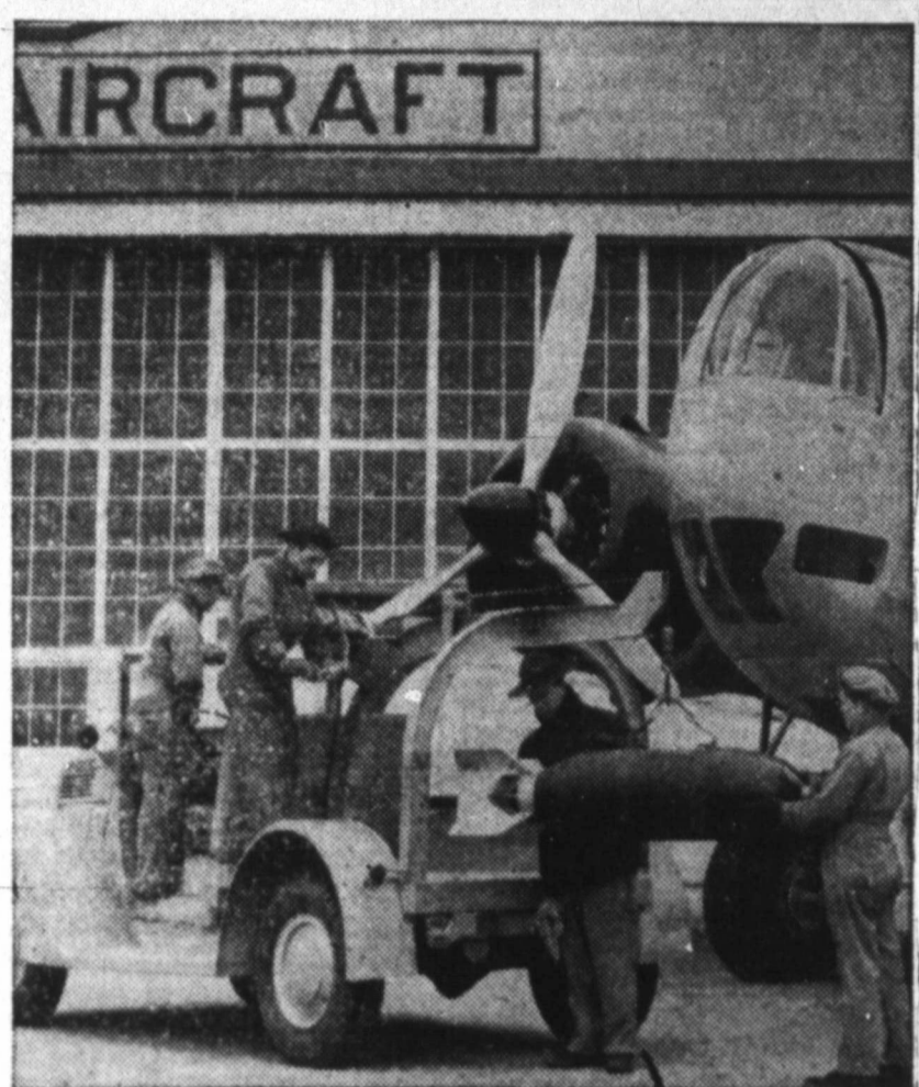
SELRIDGE FIELD, Mich.— A familiar piece of motorized equipment around U. S. Army Air Corps bases these days is this bomb service truck, shown being demonstrated near a big bombing plane at Selridge Field. Manufactured by the Ford Motor Company, the truck is rigged with special derrick and winch used to handle bombs weighing 600 to 1,200 pounds. The bomb in the photo is a dummy 600-pounder used for training purposes.
