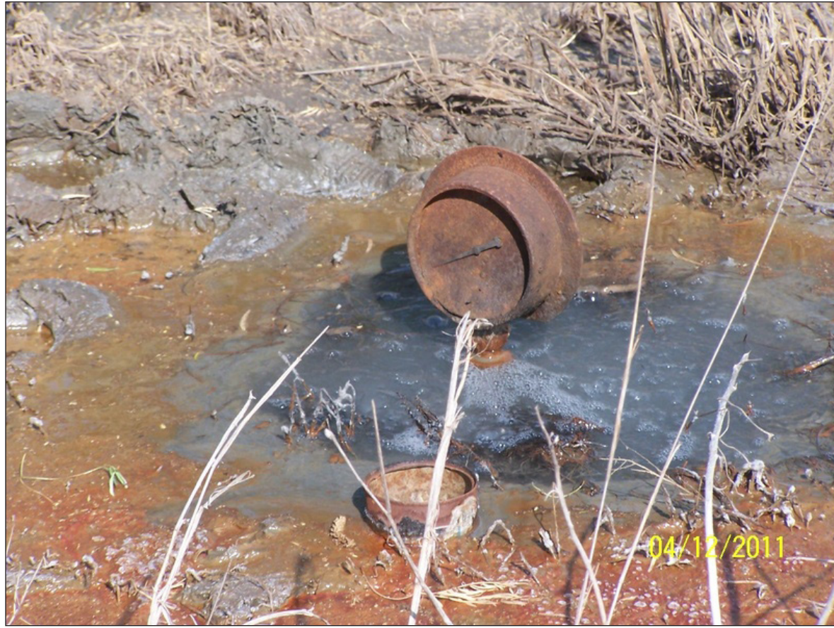
A 2011 IMAGE of the Mogford oil well well, which spewed hydrocarbons onto ranchland in Dimmit County. Some experts linked the "breakout" to nearby oilfield waste injections.
