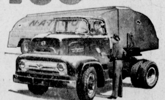
Ford F-900 with 212-h.p. V-8 has 4-barrel carburetor and dual exhausts to give you power when you need it.
