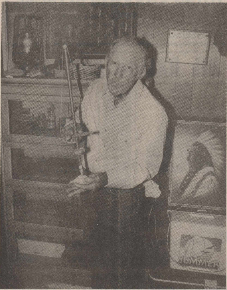
J. D. KILGORE demonstrates a drill he made after seeing Indians in New Mexico use similar ones. The drill is used for making holes in beads and for starting fires, Kilgore explains. photo by Scotty Moore
