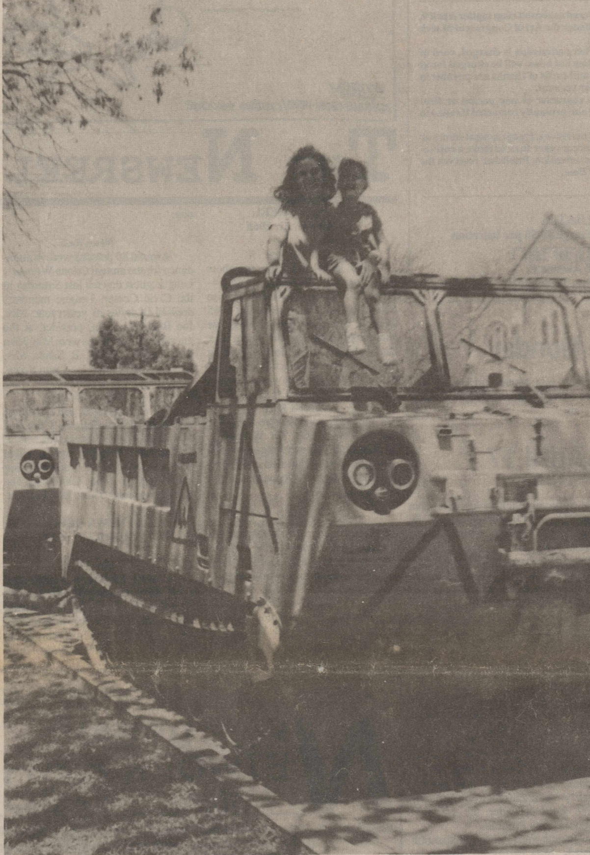
RIDING HIGH IN THE SADDLE -- Adrian Cook and daughter Danielle pose in one of Ozona Volunteer Fire Department's new track vehicles. The two vehicles were purchased from the the government surplus stockpile and will be converted with 1200 gallon water tanks and pumps to be used on range and grass fires. The vehicles will scoot along at 30 miles per hour and hold 100 gallons of fuel. In case of fire the vehicles will be transported to the scene via flat bed trailer.
