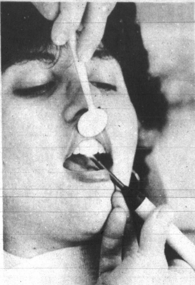
"YOU LIGHT UP my mouth," is the song this woman might sing to her dentist. That is, she might if his "optic transilluminator" were not in her mouth. The device shines an ultra-high intensity light through teeth to provide information even an X-ray cannot. The transilluminator may soon help examine the mouths of dental patients across the nation.
