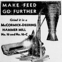
The No. 10-C Hammer Mill with feed conveyor. Note the adjustable gate at the feed throw of the conveyer.
