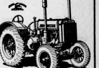
THE JOHN DEERE MODEL D TRACTOR Noted for its simplicity and power. Has only two cylinders and burns low cost fuel. Numerous less working parts to wear than most tractors, and all in dust-proof case. Takes the big jobs easily. Come in and let us explain fully its merits.
