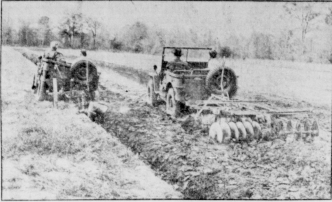
Tests at the Department of Agriculture's Tillage Machinery Laboratory, Auburn, Ala., show what jeeps can do in plowing a field and preparing the seedbed. Post-war salvage uses for the versatile blitz-buggies are being considered.
