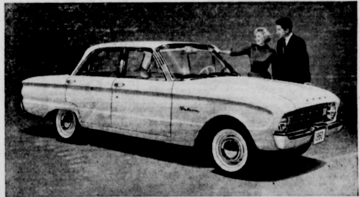
The Ford Falcon, first of America's new-size cars, represents a "breakthrough" in automotive design that may materially alter the future of the automobile industry. The Falcon Fordor shown here is more than two feet shorter and three-quarters of a ton lighter than a standard 1959 Ford. Yet, the Falcon is a six-passenger car, with interior roominess approximating that of standard models.
