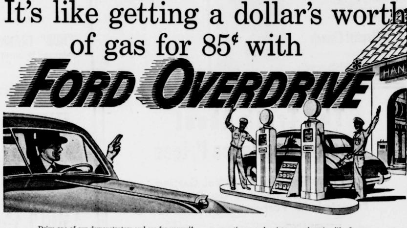
Drive one of our demonstrators and see for yourself how Ford Overdrive smooths your ride. Your engine speed actually drops 30% without any drop in road speed. For example, while your car's road speed stays at 50 m.p.h. your engine speed drops to 35 m.p.h. in Overdrive. This actually adds to engine
