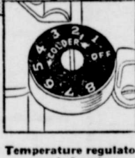
Temperature regulator speeds freezing
