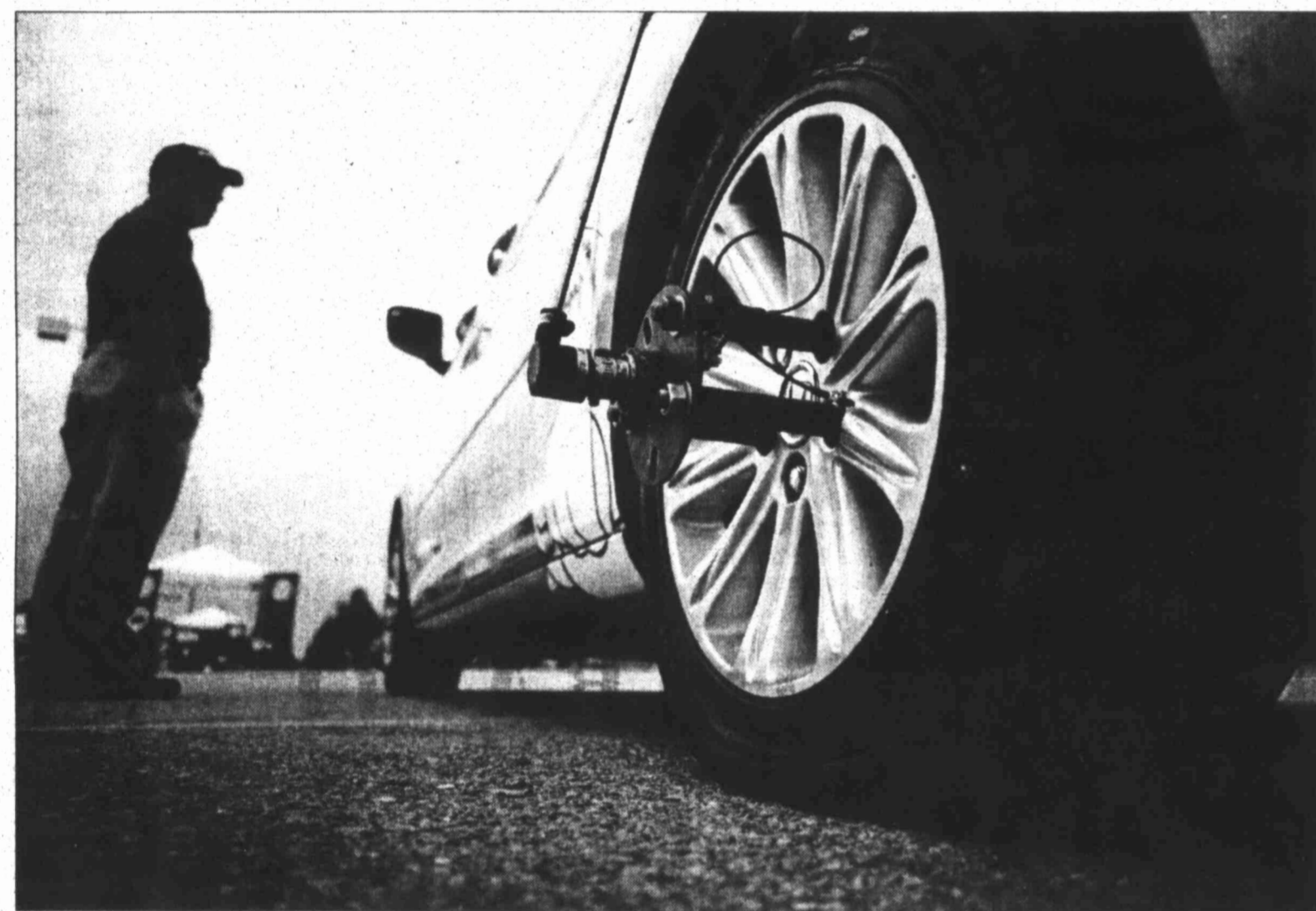
Michelin demonstrates its PAX run flat tire technology in Plymouth, Mich., which allows drivers to continue to drive even if they have a flat.
