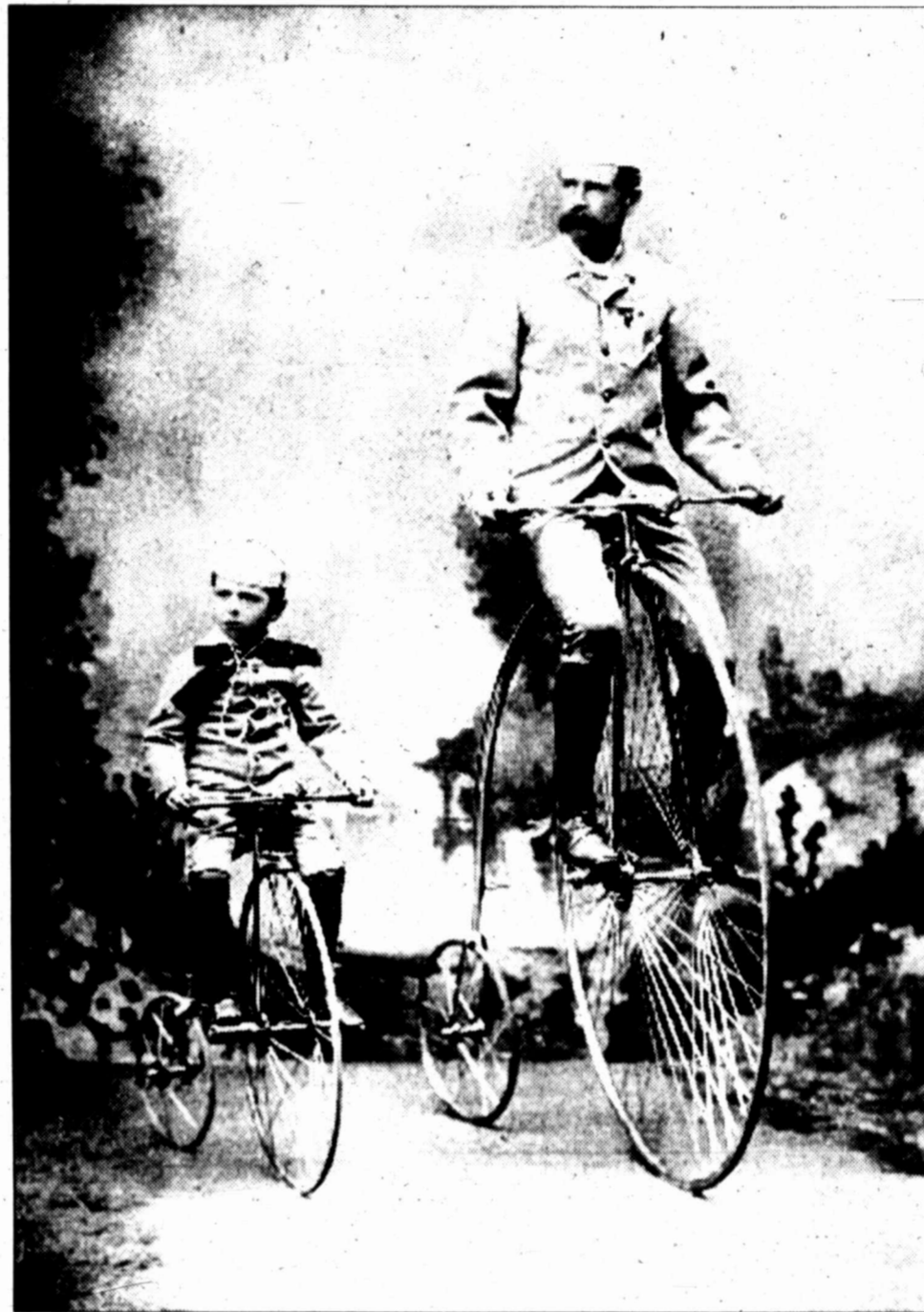
The 1882 Columbia Expert's pedals were attached to its huge front wheel, which was made of solid rubber with long spokes. Although this made for a ride smoother than on earlier cycles, the bike was really dangerous.
