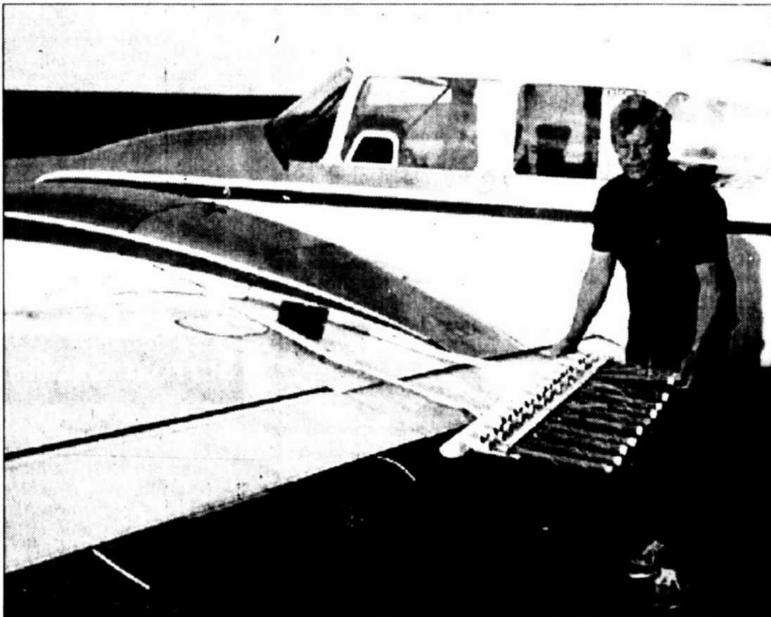
Ray Pat Jones, meteorologist for the Colorado River Municipal Water District, demonstrates how a rack of 12 silver iodide flares fits on the wing of the district's twin-engine Piper Aztec weather modification plane. The plane can carry two racks of the flares on each wing. Smoke from the flares affects the freezing temperature of water inside clouds, which increases rain output of clouds already prone to rain. The CRMWD's weather modification program is the oldest in Texas, dating back to 1971.
