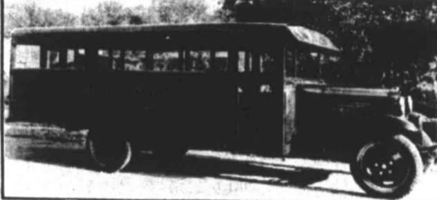
This 1933 model has a "Super Safety" metal body. Wooden buses caught fire easily, so by 1935 all buses were being built of metal. During the 1940s, few school buses were built because of World War II. After the war the number grew. Many schools were consolidated or merged. Kids were carried from rural areas to county and city schools.
