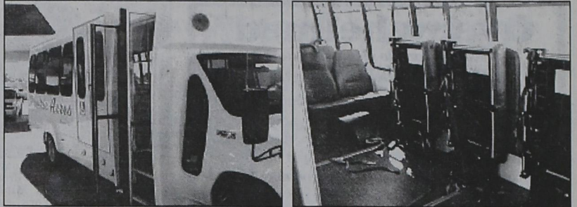
INSIDE & OUTSIDE the new Prairie Acres van purchased through a grant from TxDOT. The seats at right raise to allow wheelchair tie-downs.
