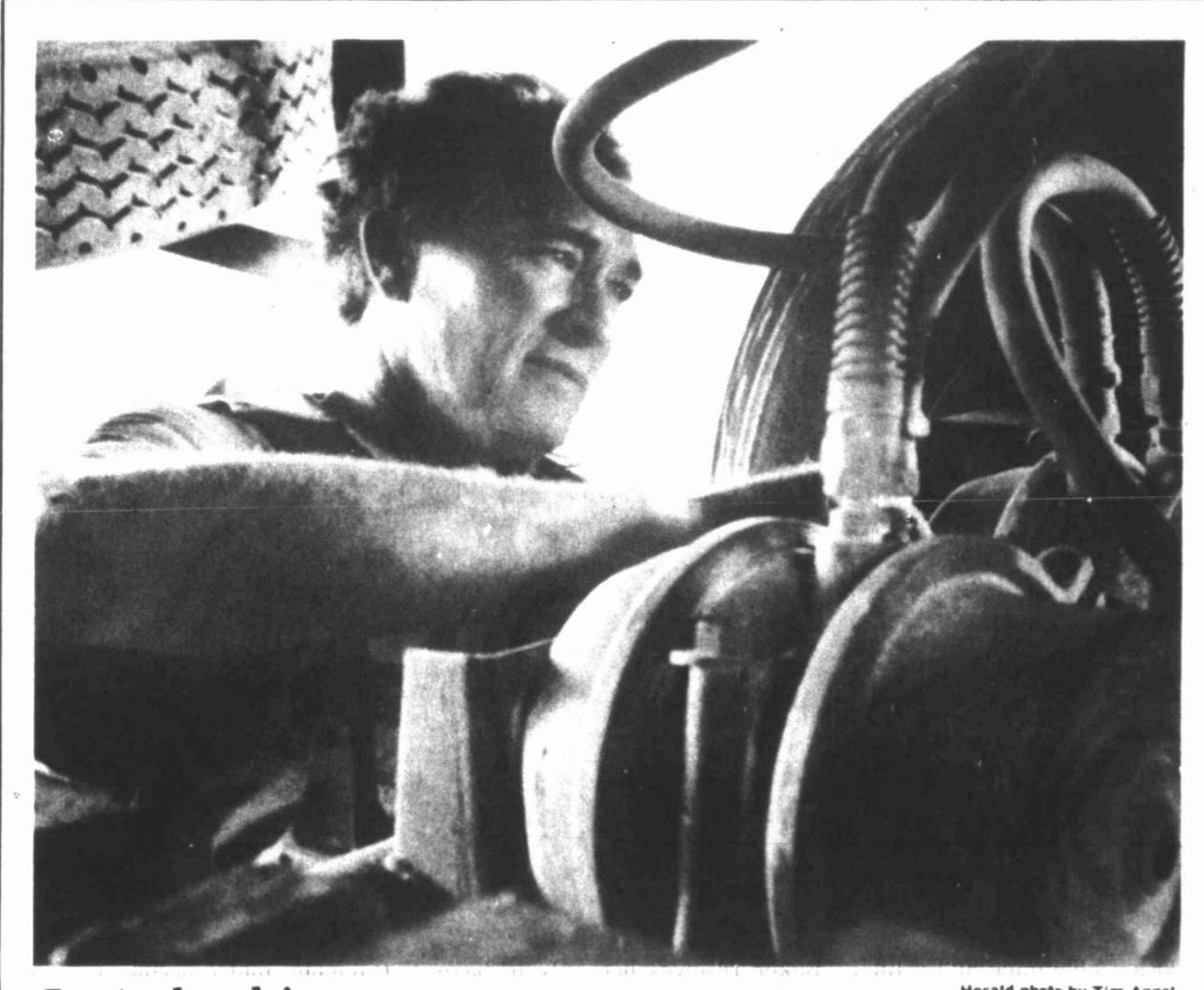
Just checking Texas Department of Public Safety license and weight trooper Donnie Gilbreath checks the brakes of a truck trailer Wednesday evening at the department's hangar in the airport. In a continuing operation, the DPS checks between 80-100 trucks per month. Herald photo by Tim Appel
